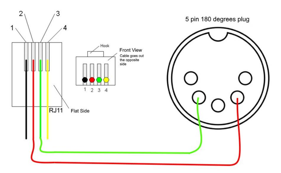
The typically RED and GREEN wires from the RJ11 plug (pins 2 & 3) are to be connected to the DIN plug's pins 4 & 5, polarity does not matter.
